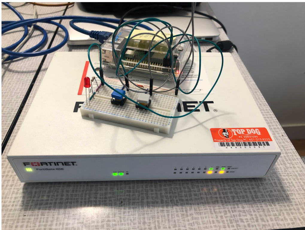
Figure 6.6: Complete setup with firewall, Pi, and components.
